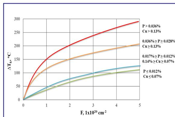
Fig. (1): Irradiation embrittlement of WWER-440 RPV surveillance specimens at high neutron fluence.
