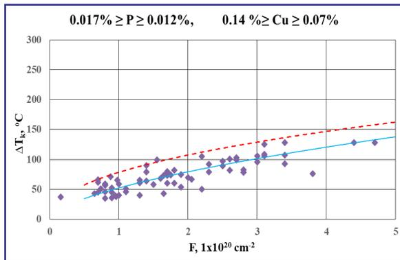
Fig. (3): Irradiation embrittlement of WWER-440 RPV “almost clean” steels at high neutron fluence (average increase, upper limit of 95% confidence interval).
