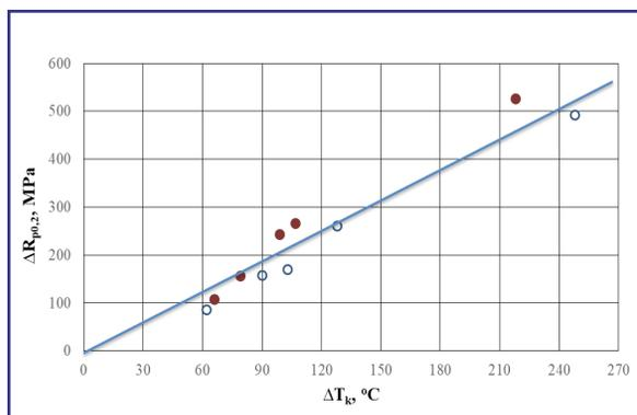
Fig. (5): Correlation of  $T_k$  shift and yield strength increase for steels with low P and Cu contents ( $\circ$  – base metal,  $\bullet$  – weld).
