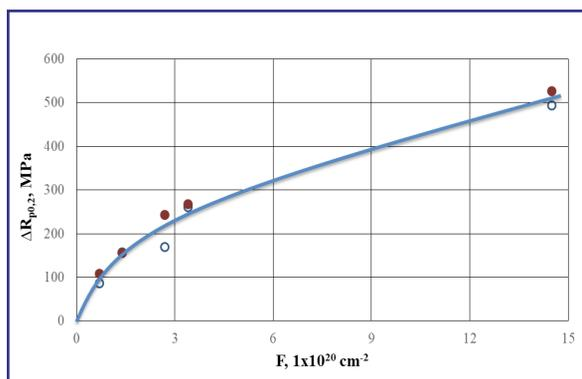
Fig. (4): Dependence of yield strength increase versus neutron fluence ( $\circ$  – base metal,  $\bullet$  – weld).
