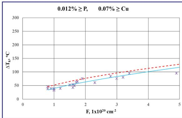
Fig. (2): Irradiation embrittlement of WWER-440 RPV “clean” steels at high neutron fluence (average increase, upper limit of 95% confidence interval).
